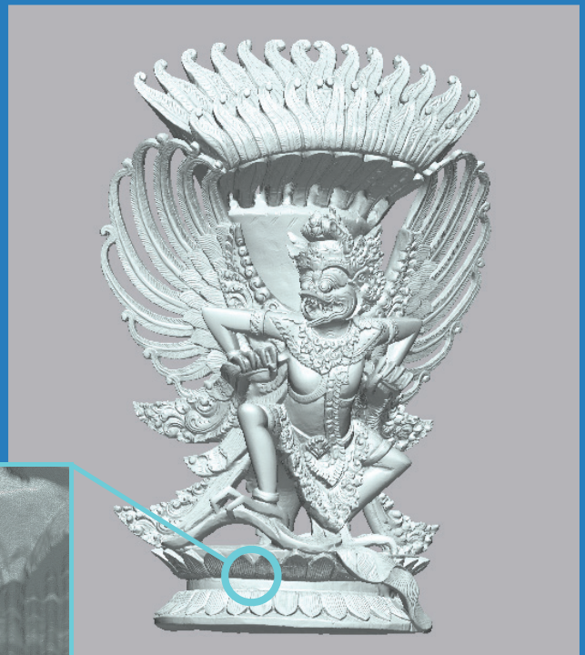
HD Scan mode with high detail function of EinScan Pro 2X 2020 (Res: 0.2mm)
