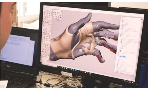
OT4 models the required splint digitally and manufactures the device with a 3D-Printer
